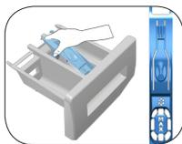
Clean the detergent drawer at regular intervals (every 4-5 washing cycles) as shown below in order to prevent accumulation of powder detergent in time.
